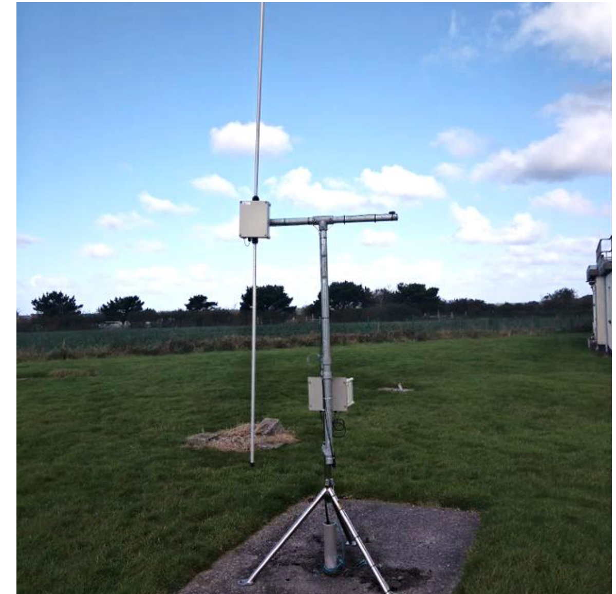
Antenna and amplifier from the UK Met Office LEELA lightning detection system.
