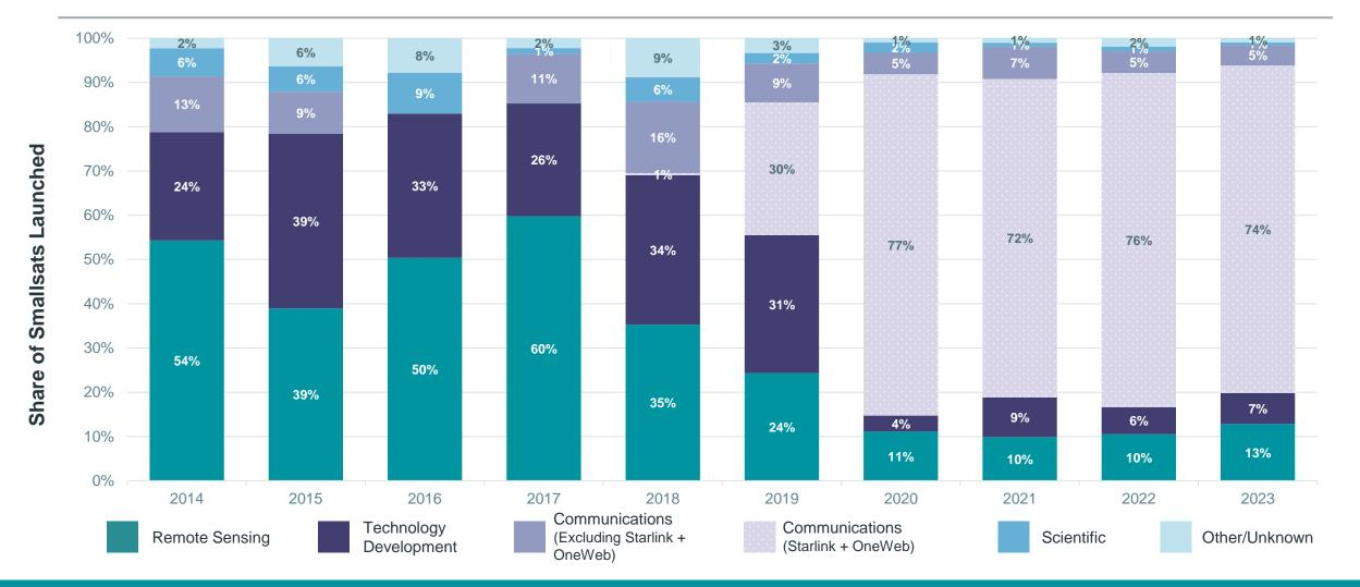
Communications satellites constitute the largest share of smallsats in 2023. Relative share of remote sensing and technology development smallsats has decreased due to launch of LEO communication smallsats
